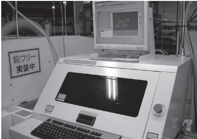
Fig. 6: Solder paste printing inspection device
